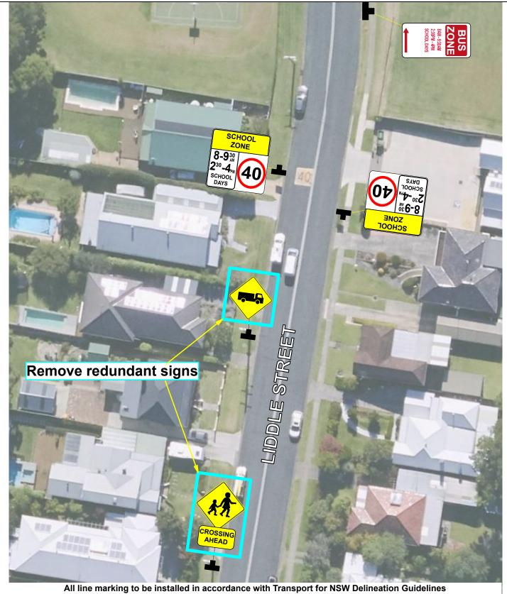
All signage to be installed in accordance with AS1742.2
