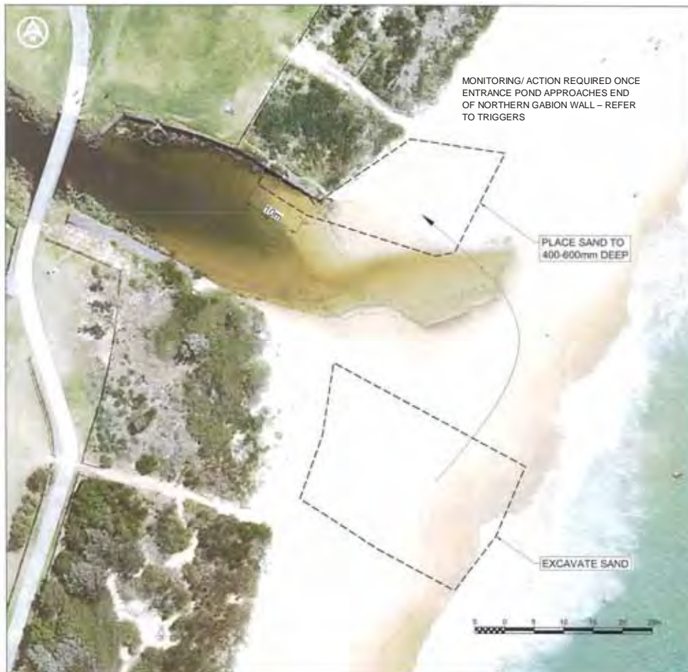
Figure 10 Typical Sand Relocation for Case 1 or Case 2
