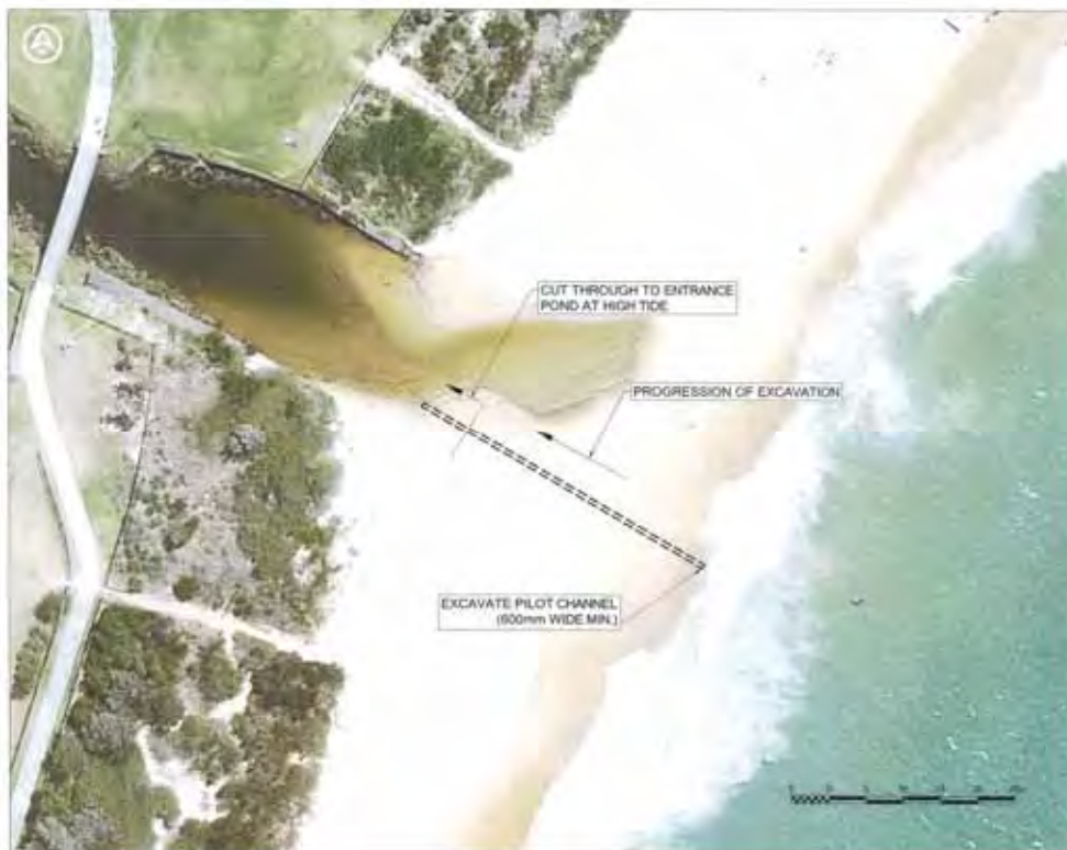
Figure 11 Typical Mechanical Breakout for Case 2
