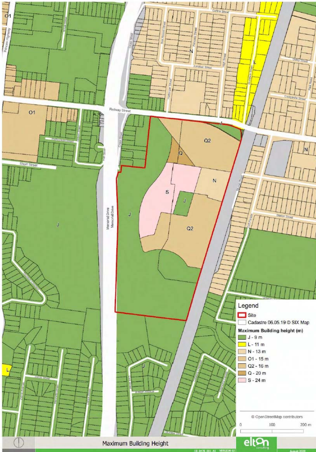
Figure 15 Height of buildings based on current definition
