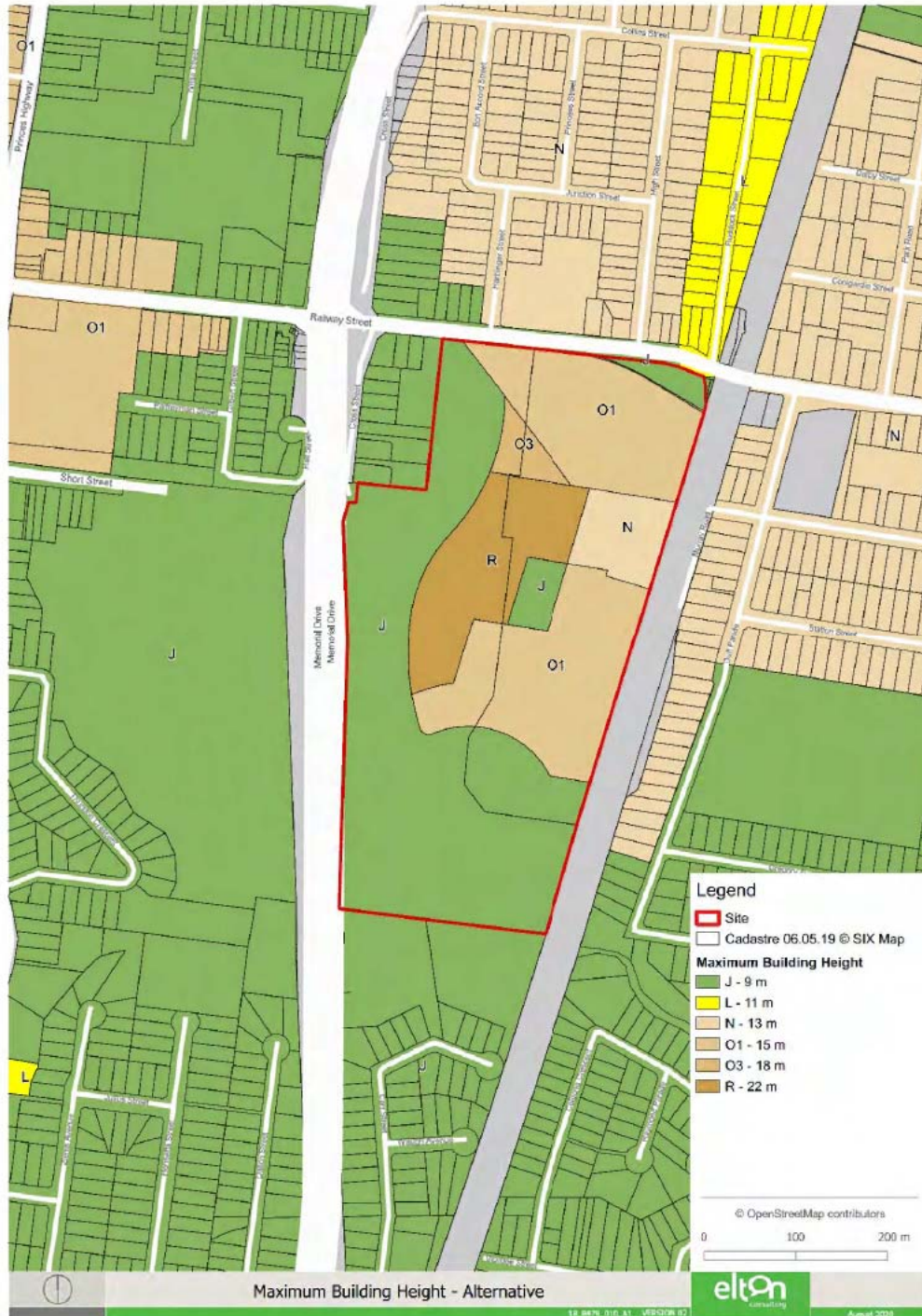
Figure 16 Proposed height based on the alternative height definition
