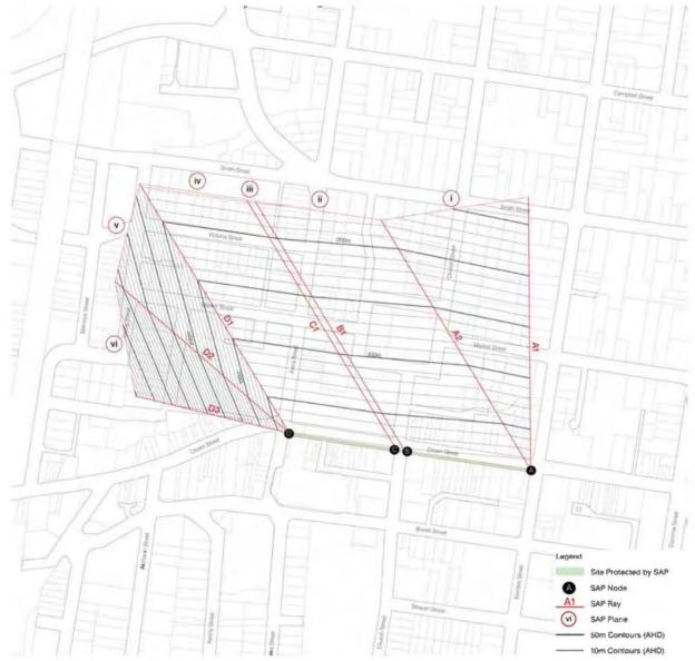
Figure 21: Crown St Mall Sun Access Plane
