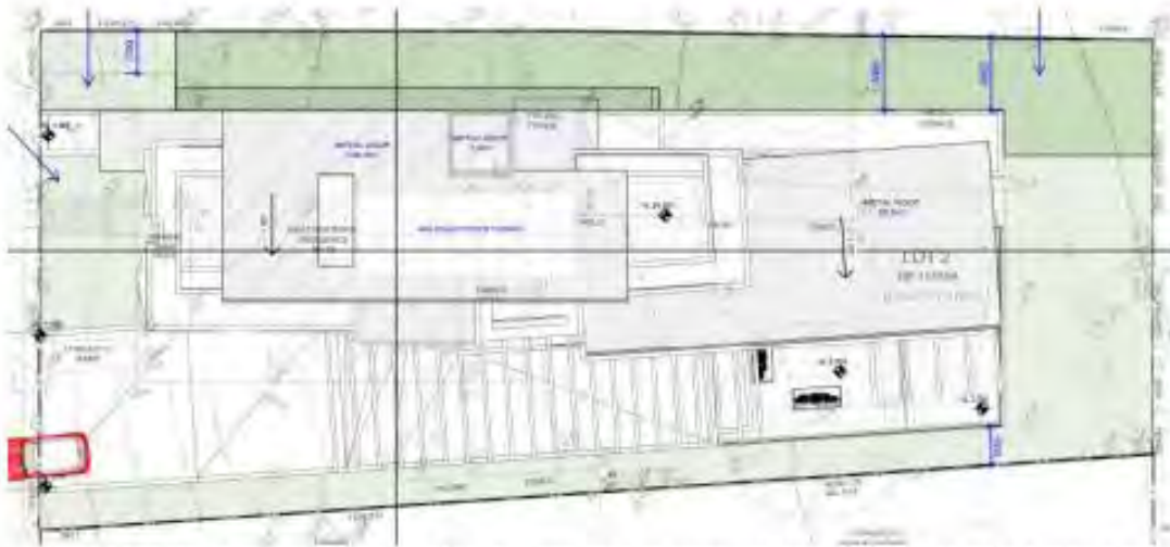
Figure 1 Site Plan showing the breakup of the building into two wings and the setbacks achieved to buildings on adjoining sites
