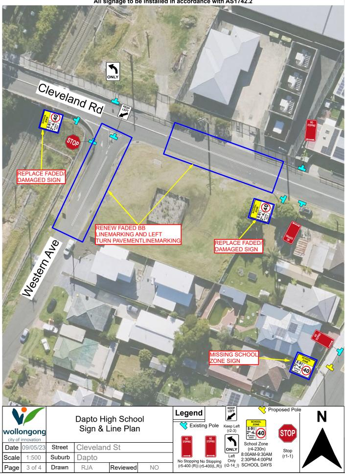
All line marking to be installed in accordance with Transport for NSW Delineation Guidelines All signage to be installed in accordance with AS1742.2
