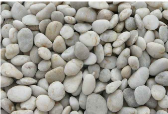
PF | WASHED RIVER PEBBLES TO ROOF BALLAST FINISH
