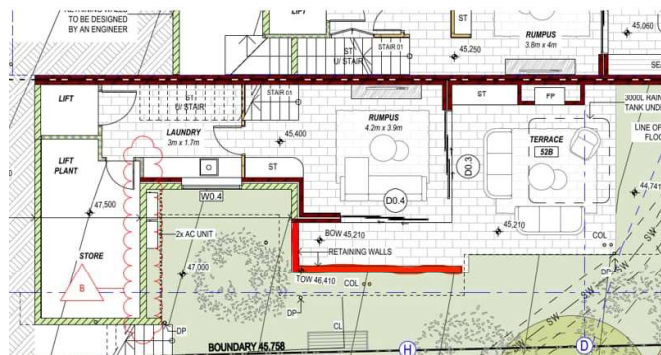
Figure 8: Extract of Lower Ground Floor Plan showing non-compliant retaining wall in red.
