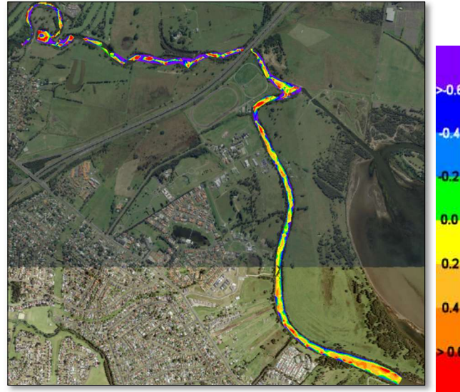
Figure 26: Mullet Creek difference plot between 2008 and 2022/2023 surveys – Negative values = possible erosion/deepening (data within Plan 539-1 Sheet 2).
