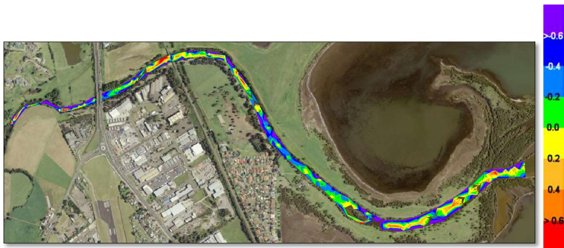
Figure 25: Macquarie Rivulet difference plot between 2008 and 2022/2023 surveys – Negative values = possible erosion/deepening (data within Plan 539-1 Sheet 5).
