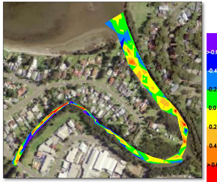
Figure 24: Horsley Creek difference plot between 2008 and 2022/2023 surveys – Negative values = possible erosion/deepening (data within Plan 539-1 Sheet 5).
