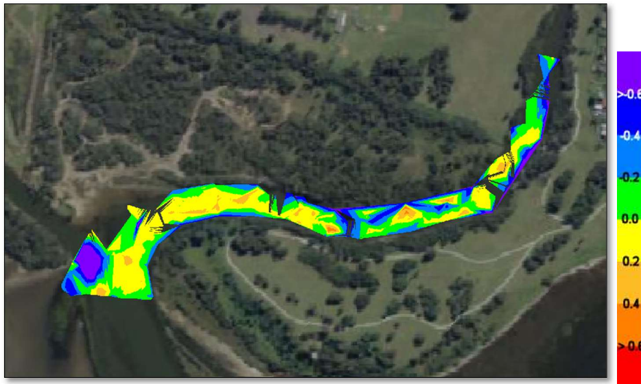
Figure 23: Hooka Creek difference plot between 2008 and 2022/2023 surveys – Negative values = possible erosion/deepening (data within Plan 539-1 Sheet 2).
