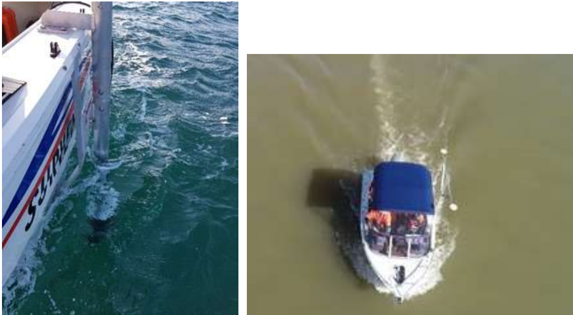
Figure 4: Survey conducted using multi beam echosounder (MBES)
