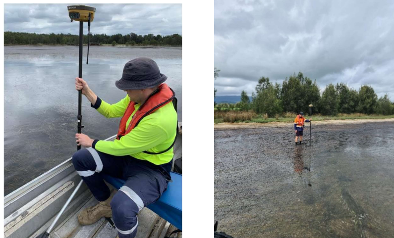
Figure 6: RTK observations by boat (left) and on foot (right)
