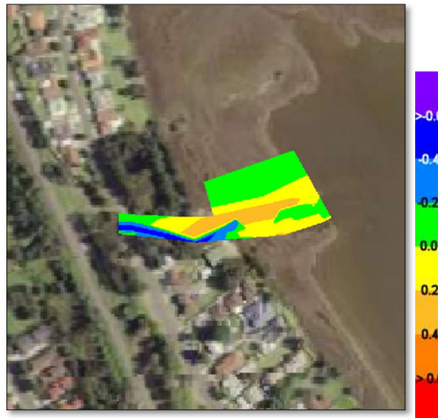
Figure 20: Albion Creek difference plot between 2008 and 2022/2023 surveys – Negative values = possible erosion/deepening (data within Plan 539-1 Sheet 4).
