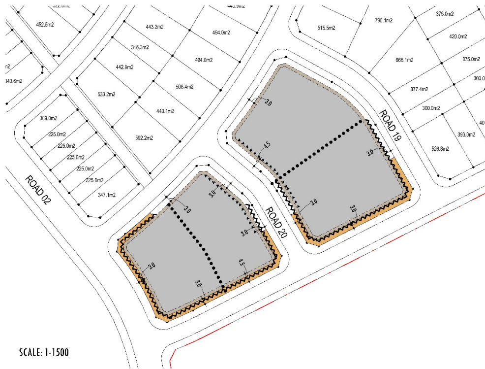
Figure 12 Schematic set out of building features interfacing with the public realm for medium density development
