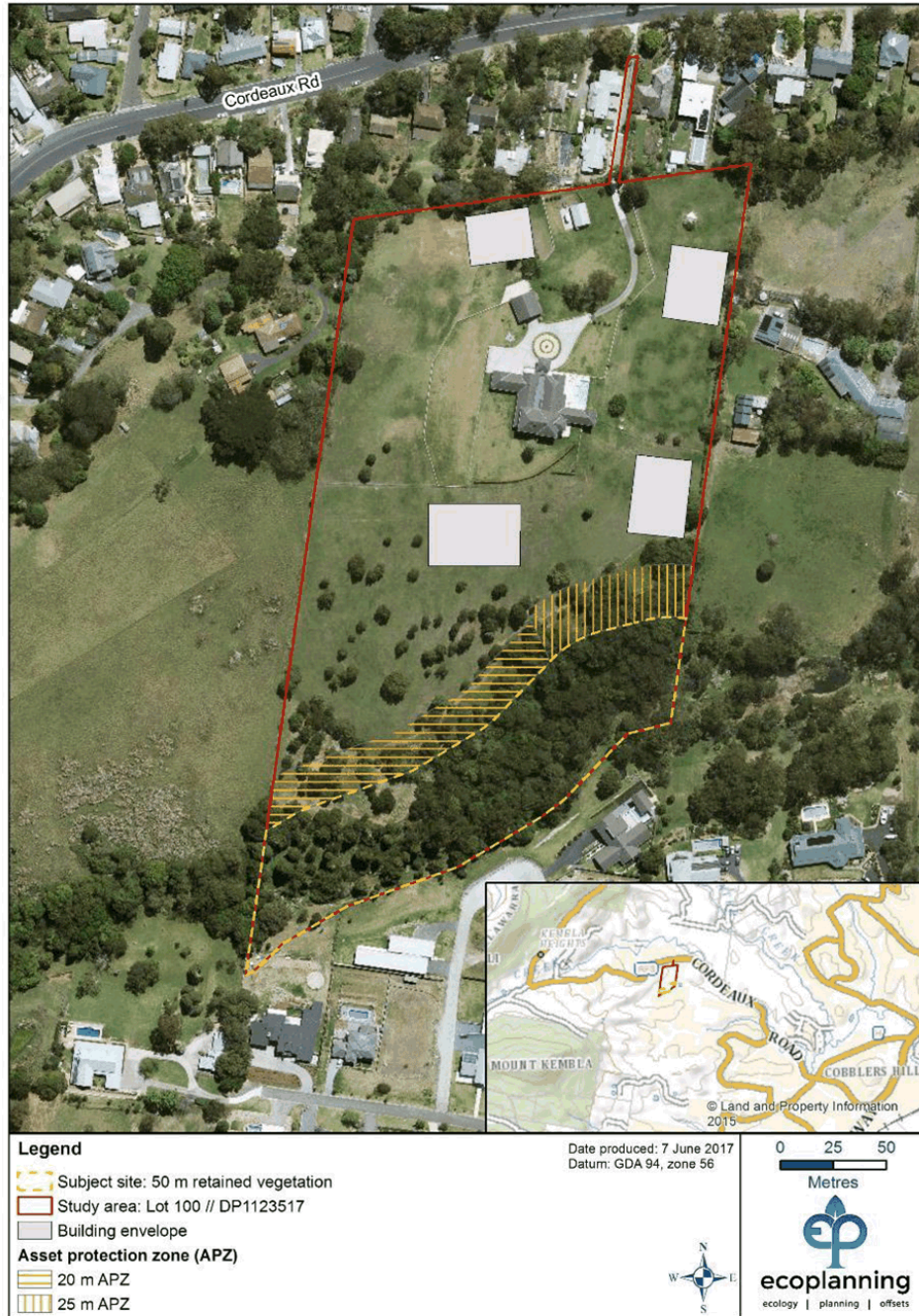
Figure 1.1: The study area and VMP subject site, including the proposed lot layout and APZs.
