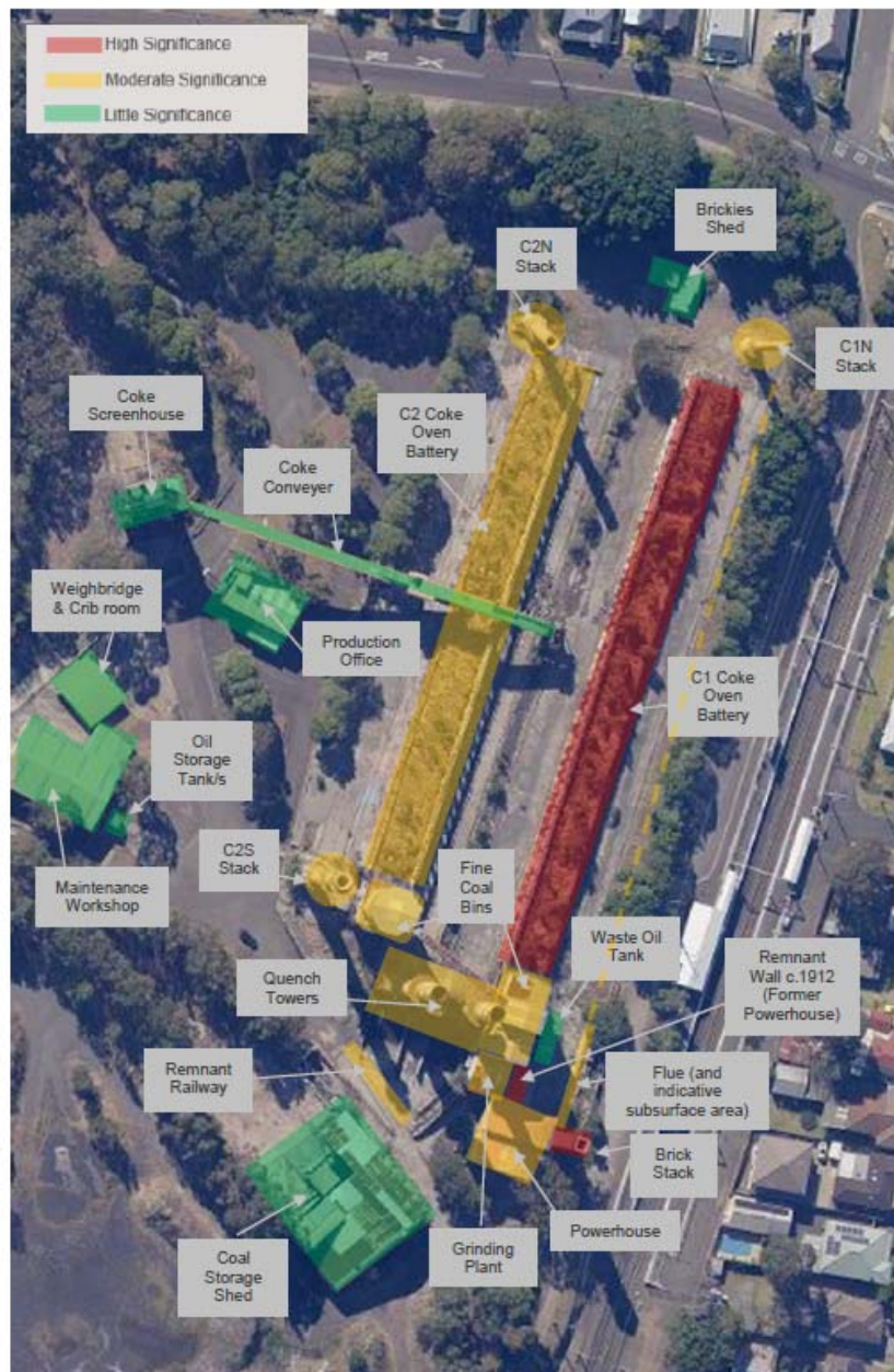
Figure 94 - Former Coke Works Significance Map - Detail
