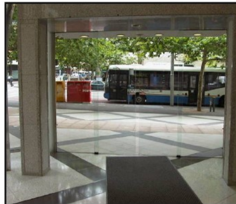
Figure 2022: (Top left) Very shiny and slippery floor surfaces which fail to meet the "R" rating, as required by AS4586 and HB197.
