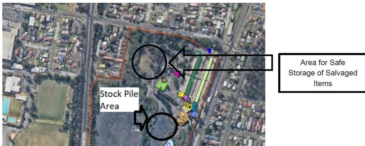
Figure 6: Salvage area as indicated in Demolition Work Plan
