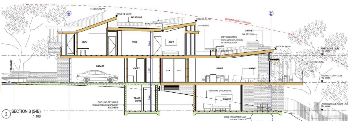
Figure 2: Extract of Section Plan prepared by MacCormick + Associates Architects showing Section B through No. 54B.
