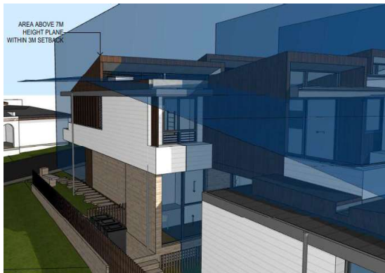
Figure 31: Extract of wall height and setback plan for eastern boundary prepared by Maccormick + Associates Architects illustrating areas above the 7m height line and within the 3m setback.
