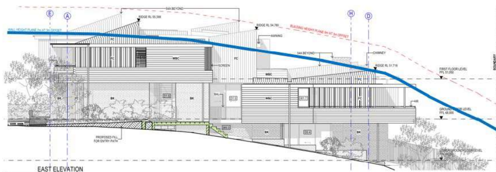
Figure 29: Extract from East Elevation Plan prepared by Maccormick + Associates Architects illustrating 7m height line in blue.
