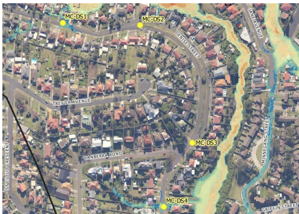
Figure 8-5 Minnegang Creek Downstream Road Overtopping Locations (with 1% AEP Risk Scenario)
