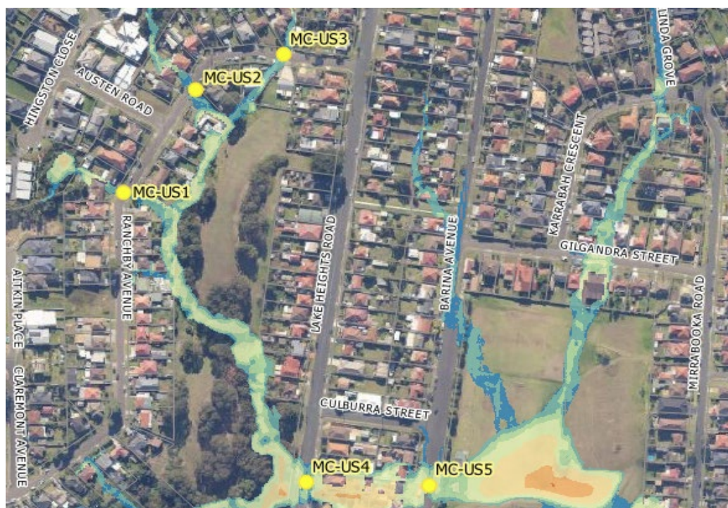
Figure 8-3 Minnegang Creek Upstream Road Overtopping Locations (with 1% AEP Risk Scenario)
