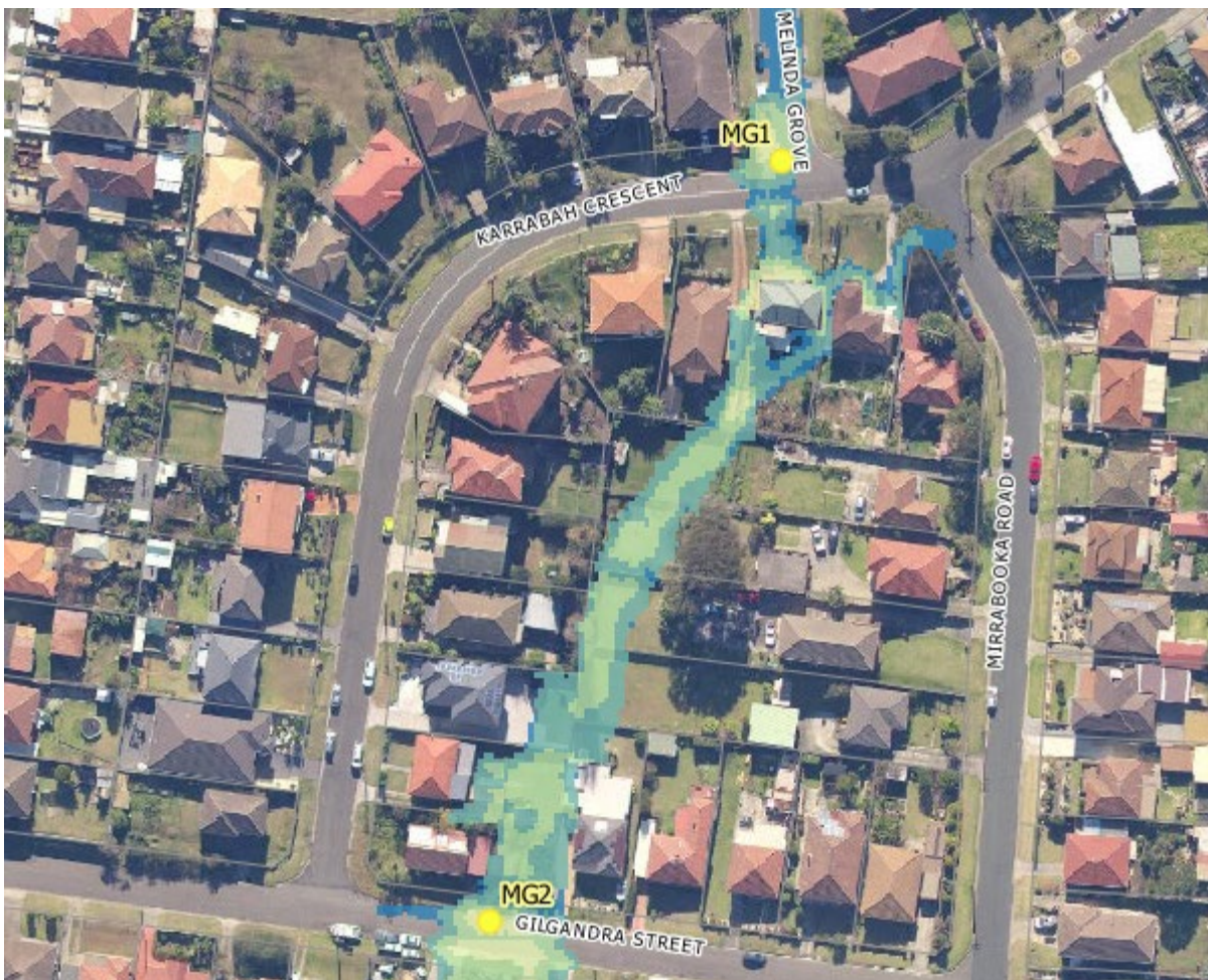
Figure 8-2 Melinda Grove Tributary Road Overtopping Locations (with 1% AEP Risk Scenario)
