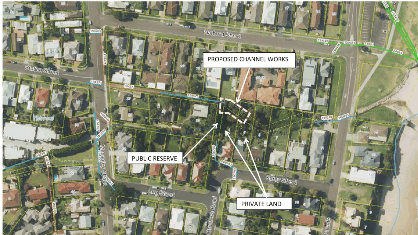
Proposed channel excavation works in Council reserve and private land. Numbered lines denote Council owned stormwater pipes.
