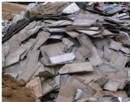
Figure 2: Bonded Asbestos Tiles
