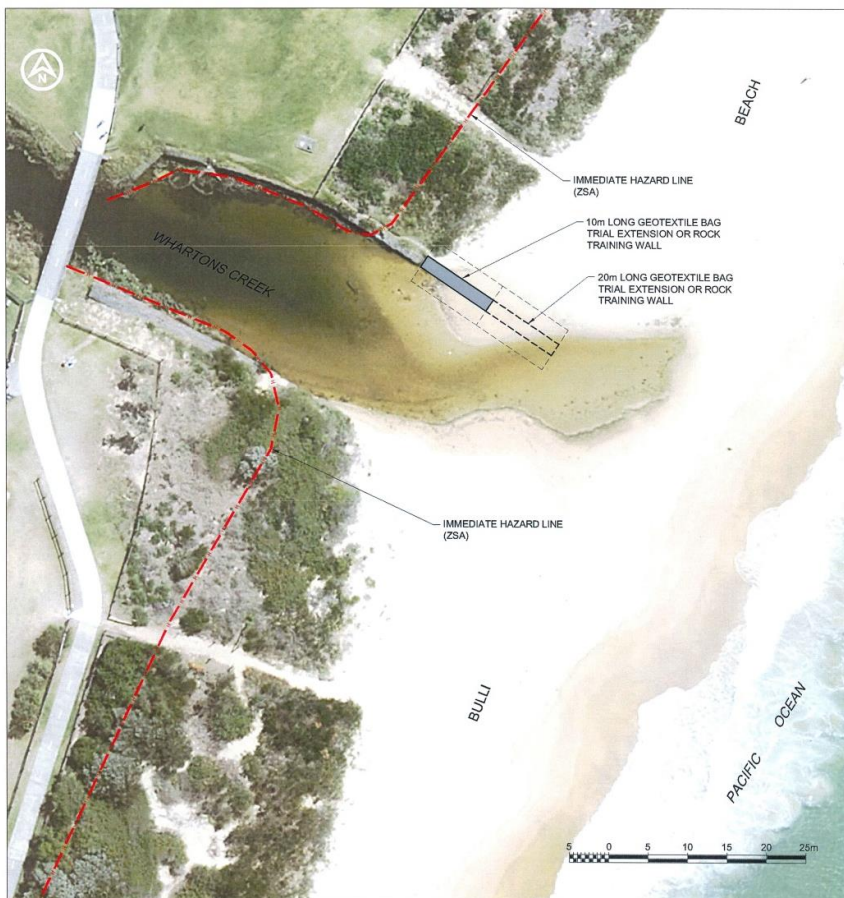
Figure 8 Training Wall Extension Concept Plan [100 year ARI immediate Zone of Slope Adjustment line shown CLT (2010)]
